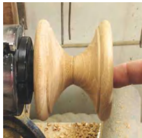
▲ Pic.15 Once you are happy with the shape, it's time to turn its twin. A good way of seeing how accurate you are is to put them 'nose to nose' like this
